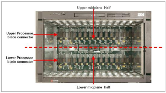
Figure 2-3 Internal picture of the upper and lower midplane of the BladeCenter chassis
